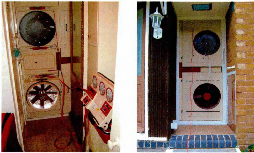
Figure 2.12: Internal and external view of blower door [Source: Sharples and Goodacre, 2004]
